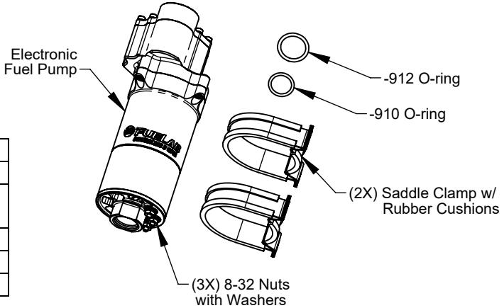
**WARNING!** Power Supply Voltage must be constant as specified in above specification. Only install fuel pump on vehicles using between 12 Volt (6 cell lead acid battery) and 24 Volt (12 cell lead acid battery) systems with or without a normal operating charging system. Pulse-Width Modulation or other means of reducing input power voltage may result in erratic or non-operational condition. Consult these instructions on using pulse width modulated signals for means of fuel pump speed control.
