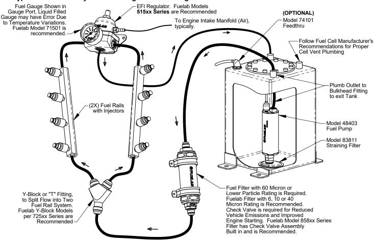
Typical EFI V-8 Fuel System Plumbing Schematic Diagram:
