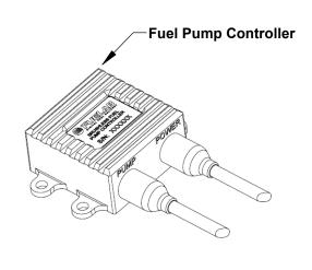
WARNING! This DC Brushless Fuel Pump Controller is ONLY compatible with 3 Phase DC Brushless Fuel Pumps without an internal electronic controller, 3 Phase Brushless Fuel Pumps feature three wires that are directly attached to the internal motor's stator windings. This controller is INCOMPATIBLE with ALL two-wire (using power and ground only for operation) systems.
