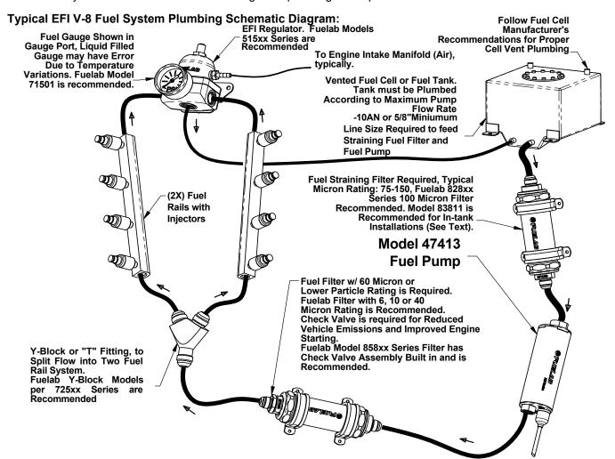
Special Note: Use in carbureted systems require a bypass return or relief valve. Do not "Dead Head" Fuel Pump.
