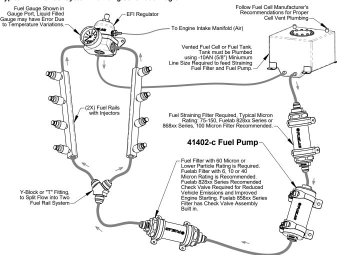
Special Note: Use in carbureted systems require a bypass return or relief valve.
