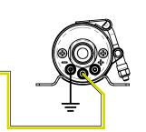
Refer to above Example 5, for use with the Fuelab Electronic Fuel Pressure Regulator, Models 52901 and 52902, that creates its own pulsed signal. These regulators automatically control the fuel pump, without the use of switching means or other components such as described in examples 2 and 3. Refer to instructions for the Electronic Regulator for proper wiring and installation.
