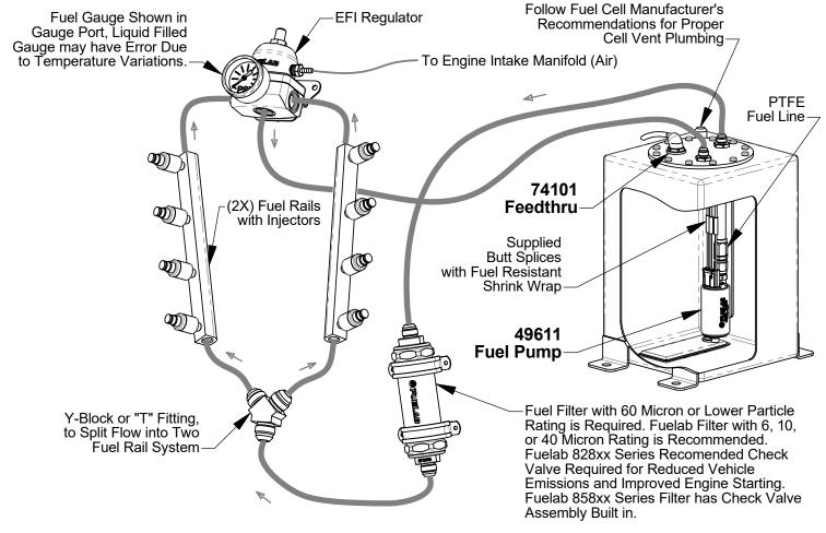
Special Note: Use in carbureted systems require a bypass return or relief valve. Do not "Dead Head" Fuel Pump.
