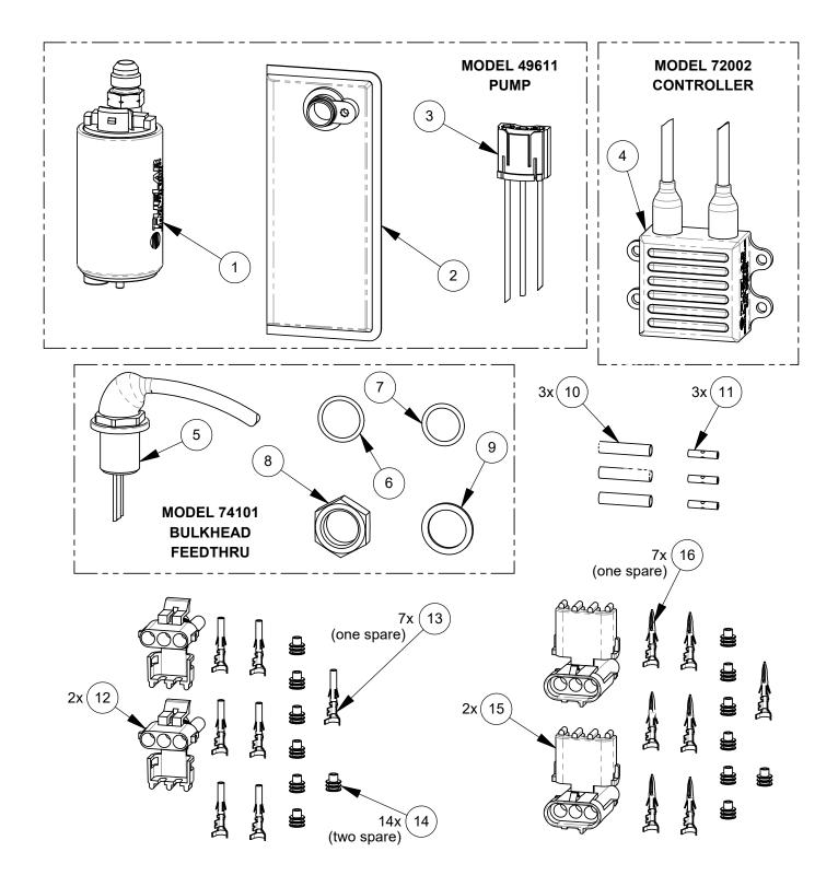
Check above diagram and list shown on previous page, to ensure no components are missing or damaged. Contact your Fuelab<sub>®</sub> distributor immediately for replacement.
