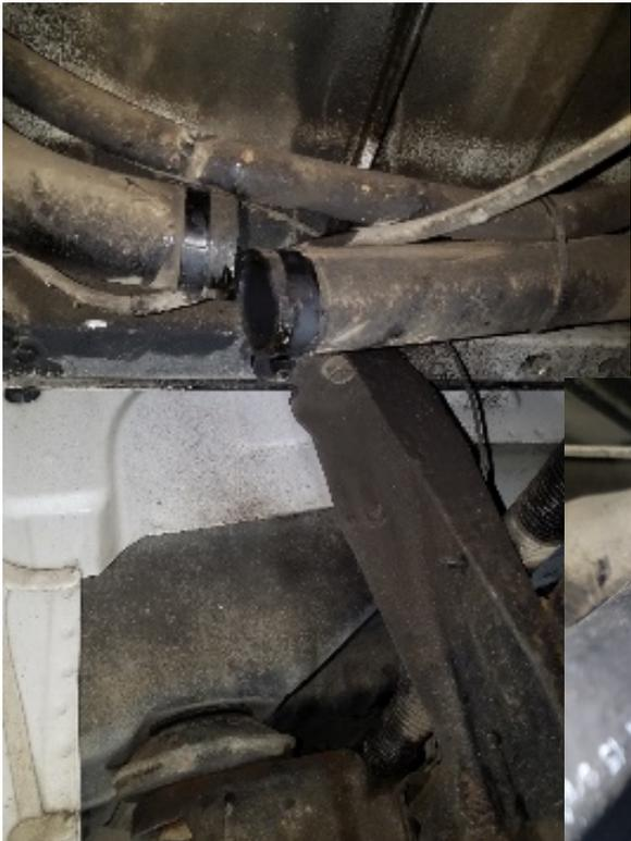
Cut filler neck line (shown left) and install filler neck adapter and clamps (shown below). Measure Distance between the filler neck QC and the pump return QC leaving enough for a smooth transition. Install one 90° QC fitting (item 4) and one straight QC fitting (item 6) and install return line section of fuel line.
