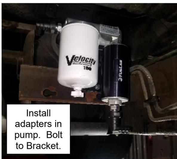
Install Male Quick Connects (Items 2 and 3) onto Lift Pump / Filtration System. **Special Note:** Each fitting being attached to the Lift Pump / Filtration System MUST use an O-ring to seal the connection against the Pump. Use small amount of oil or diesel fuel on O-rings prior to installation of fittings into pump.
