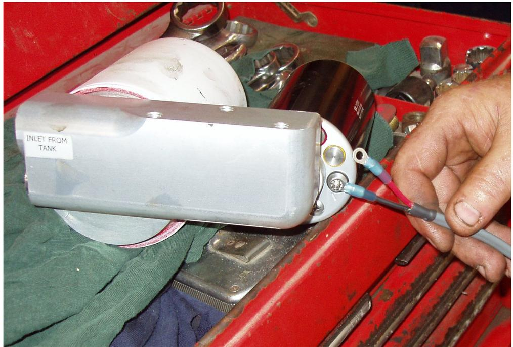
Connect the three harness wires to pump as shown, right. Route harness up to the fuse box and install the fuse tap. Install the ground wire.
