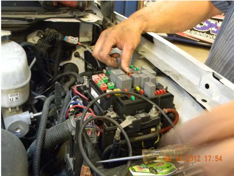
Run the wiring harness (Item 10) along the driver side frame rail and secure with Cable Ties (Items 8).
