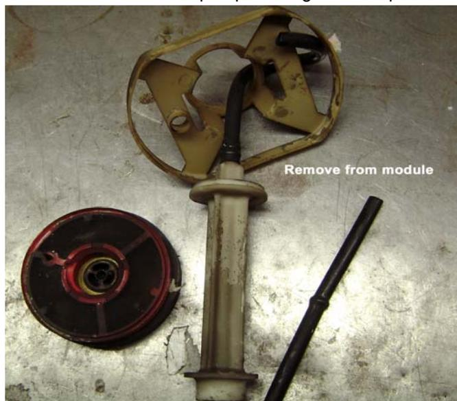
fuel tank level sender. Remove other unneeded components within the fuel tank module as well including additional straining filters (such as shown in the photo to the left).
