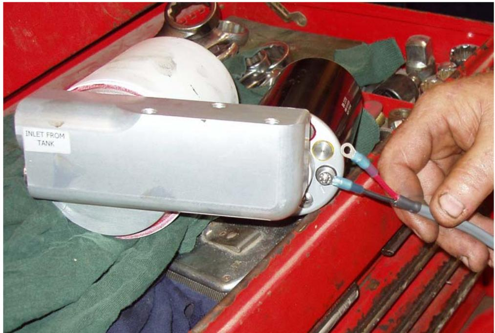
**Step 7:** The Fuel Line (item 1) and Push-lok® fittings (items 2, 3 and 5) are very tight. Use a small amount of oil on the fittings and use a heat gun to soften the fuel lines slightly, to fully seat them.
