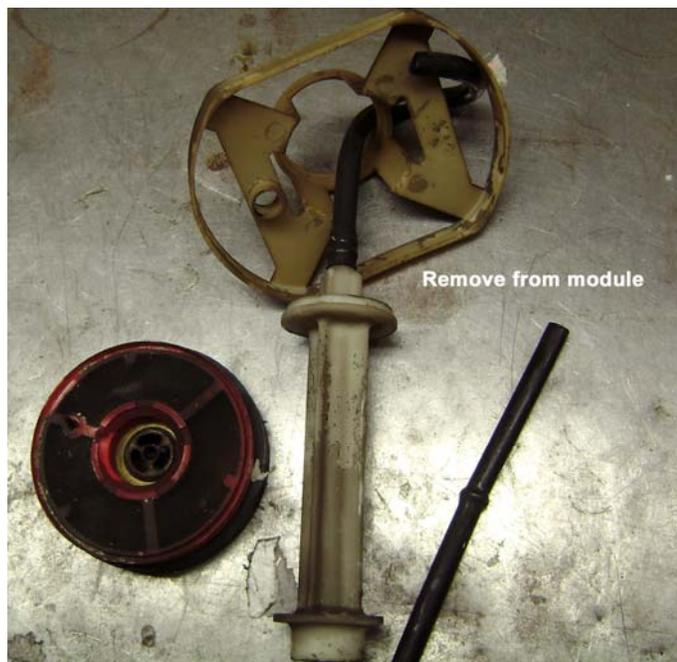
Remove and discard the original in-tank fuel pump from the fuel tank module (if present), and wire tie any wiring from pump, to secure (wiring of fuel pump is no longer required, do not short wires together). Wiring is still required for the fuel tank level sender. Remove other unneeded components within the fuel tank module as well including additional straining filters (such as shown in the photo to the left).
