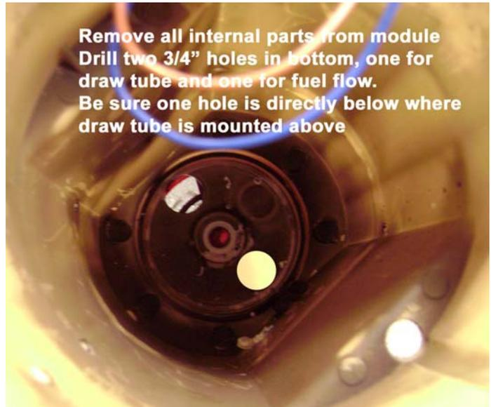
Install the modified fuel tank module (example shown to the right). Take extra care to ensure that the fuel tank level sender arm and sensor do not get damaged upon installation. Before seating the fuel tank module, ensure that the gasket seal is in its proper position prior to setting it in place. Re-attach the fuel tank module's lock ring to secure the fuel tank module back into fuel tank. Position the fuel tank back under the vehicle to begin the process of reinstallation.
