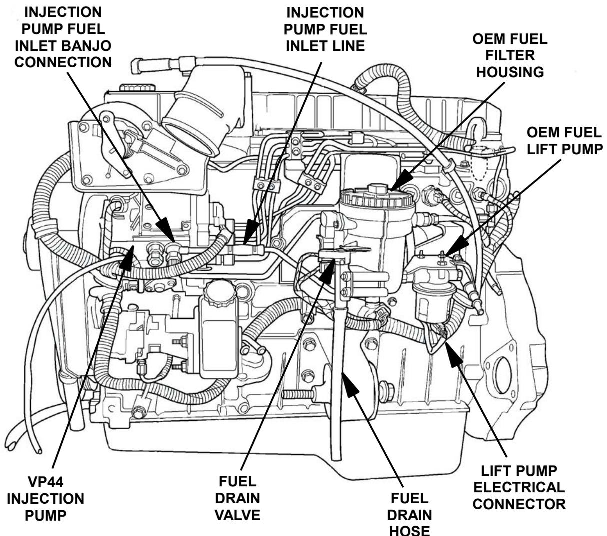
**1998.5-2002 DODGE CUMMINS TRUCKS, USING VP44 INJECTION PUMP**
